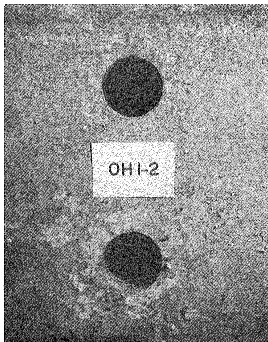
FIG. 29. Faying Surface Damage of OH1 Joint (1/16-in Clearance)
