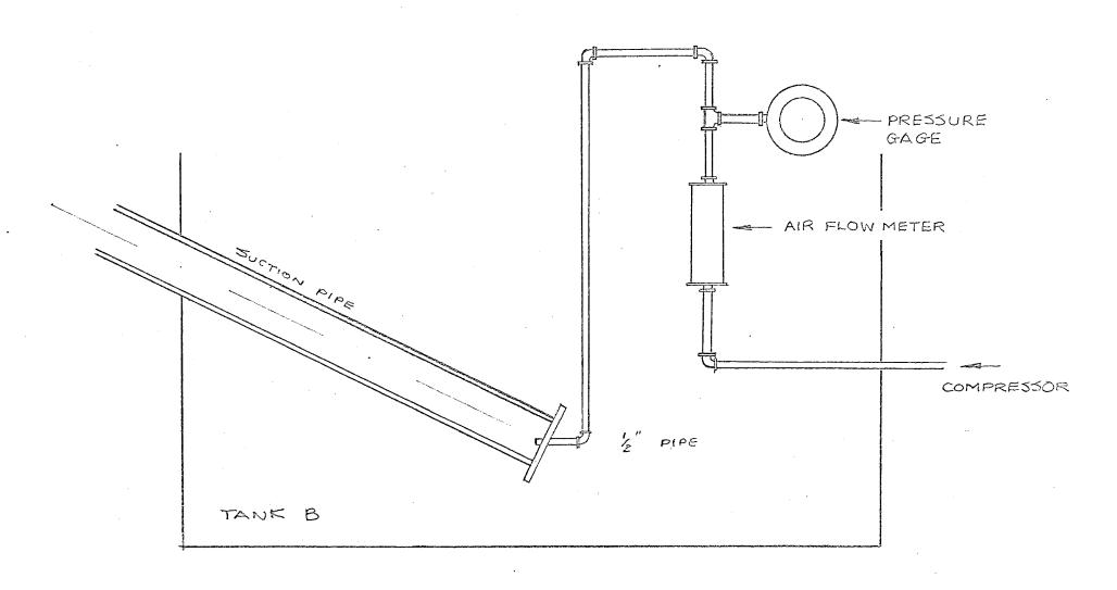
Fig. 4 Sketch of Single Port Injection System
