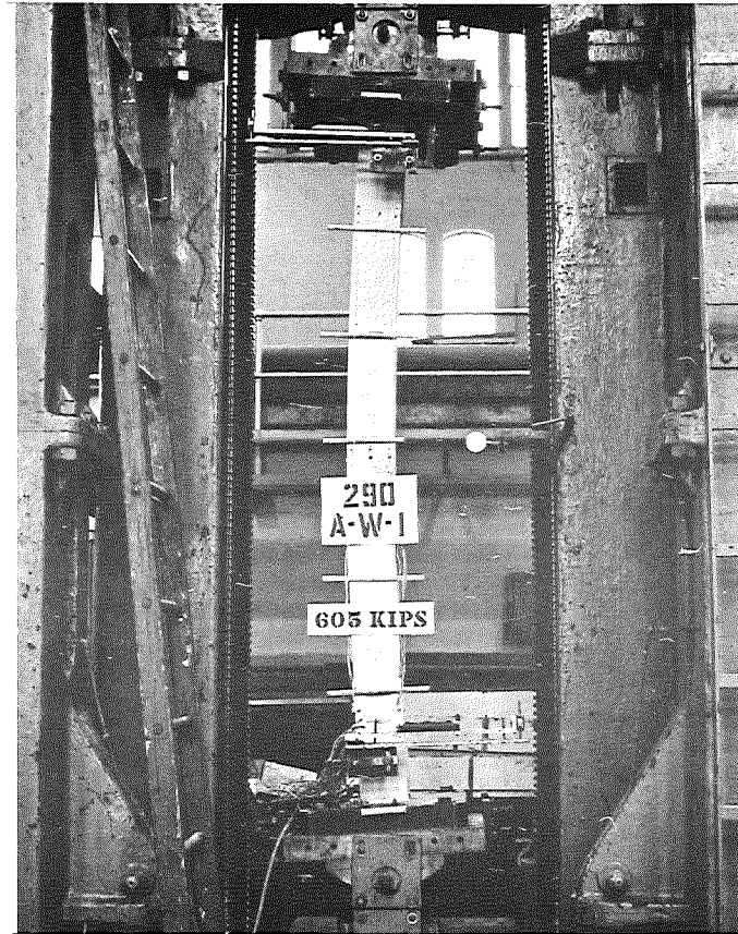
(b) Immediately After Abrupt Failure
