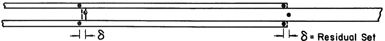
9e: Joint Under Zero Load-After Unloading
