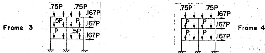
FIG. 2 LOADING CONDITION AT ULTIMATE LOAD
