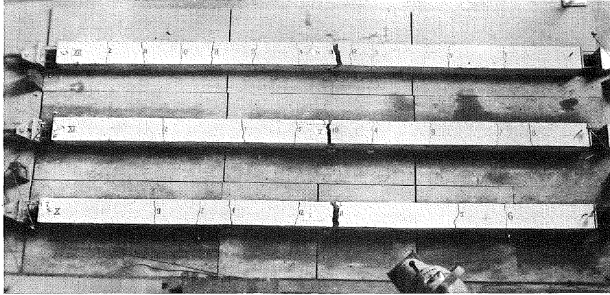
FIG. 22A - CRACK SEQUENCE IN SET D
