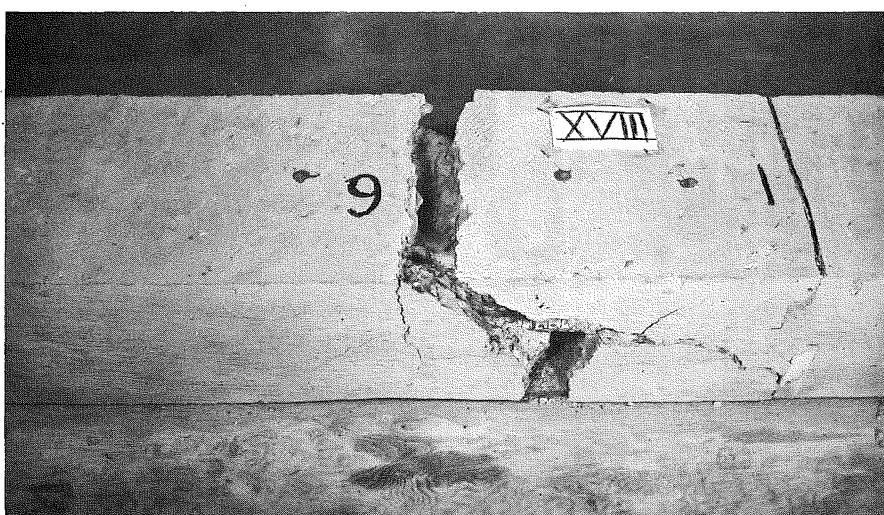
FIG. 24D - FAILURE OF SPECIMEN XVIII (SET F)
