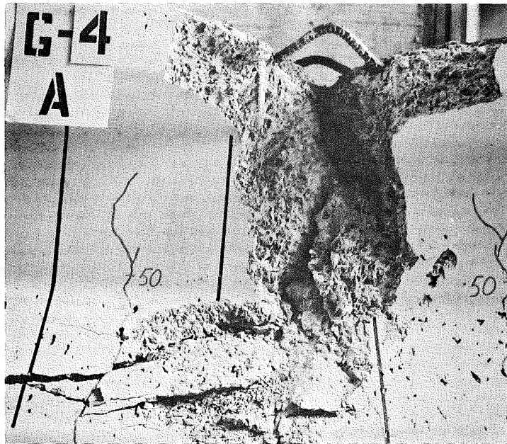
b. View of Flexural Failure Region
