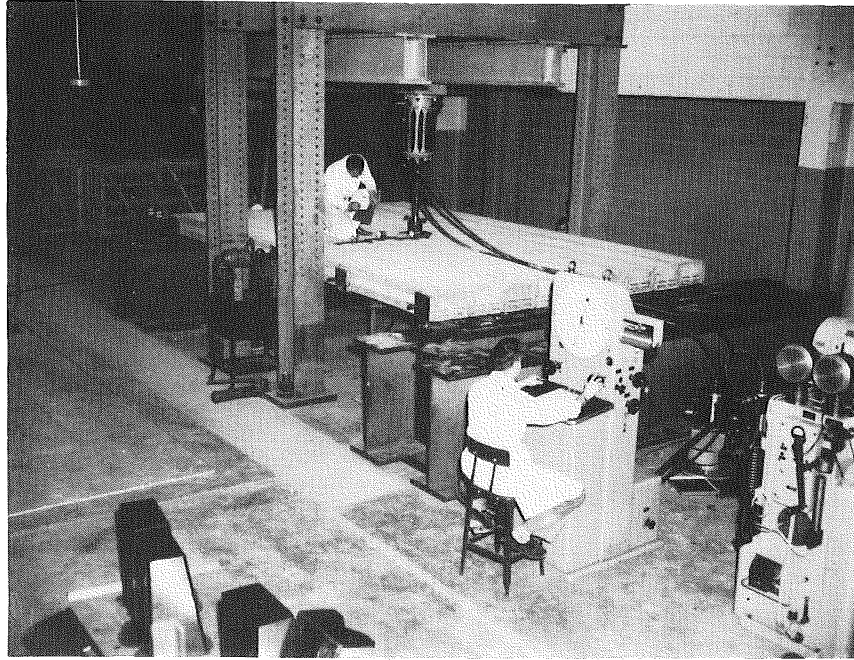
FIG. 5 TEST SET-UP OF THE LABORATORY BRIDGE
