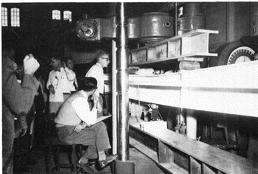
Applying load over an unsupported span too long to prevent premature buckling.....
