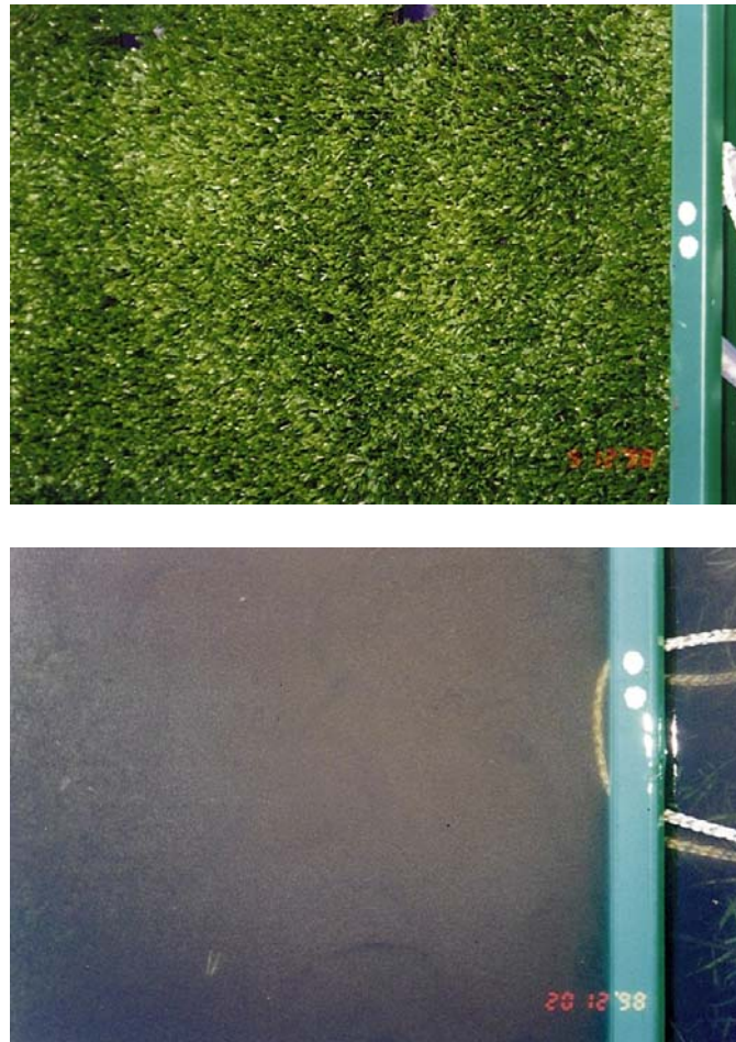
FIG. 29. One of three trays of artificial spawning substratum before (above) and after (below) its installation in Bassenthwaite Lake between 5 and 20 December 1998, illustrating the degree of the problem of the local deposition of fine sediments. Reproduced from Winfield (1999).
