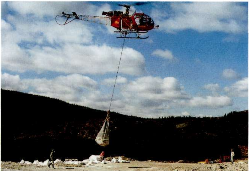
FIG. 4. Transporting bags of powdered lime by helicopter from a depot just outside the Fleet catchment.
