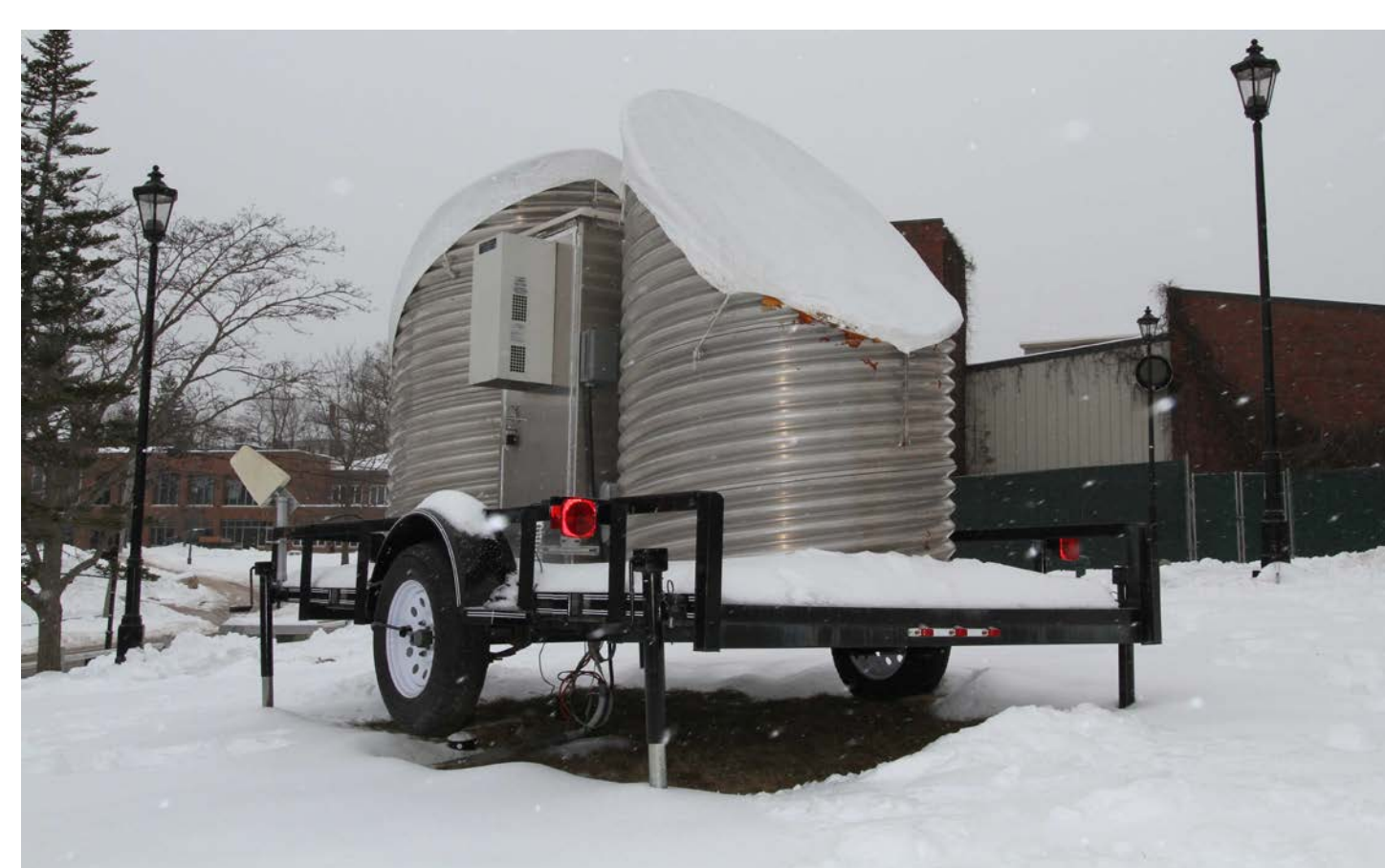
Plymouth State University's Snow-Level Radar
