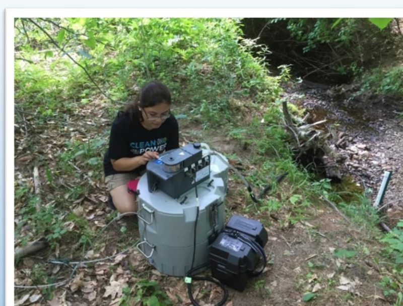
Fig 8: Setting Isco sampler to catch storm event in Livermore Cove Brook
