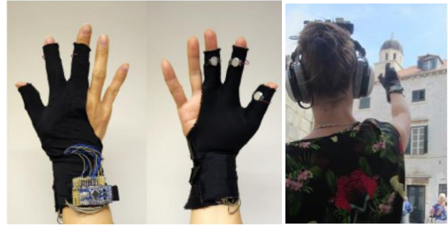
Figure 4: Left the haptic glove; and right the audio-haptic exploration, in which a user points at a POI with the haptic glove and listens the associated audio description.
