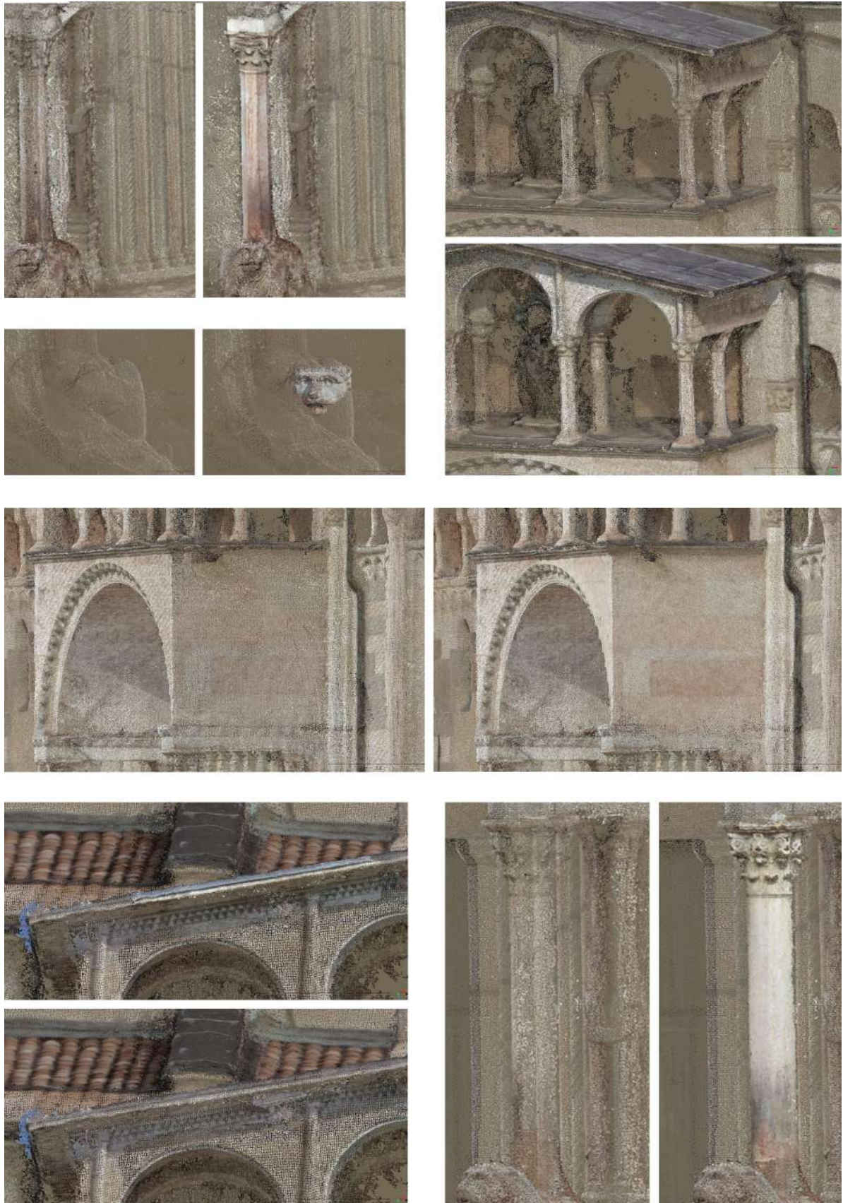
Figure 8: Single-cluster visual evaluation of the improvements in the dense point clouds obtained after the filtering procedure. Dense point clouds computed for each cluster show a general improvement of results, with much denser point clouds, less noise and a higher definition of the architectural details.
