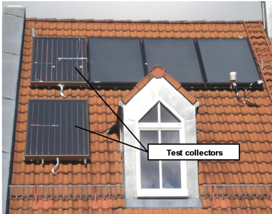
Figure 2.3: Part of the collector array with the system integrated test collector (top, left) and the test collector which is permanently stagnating (bottom, left; Reiter et al. 2012)
