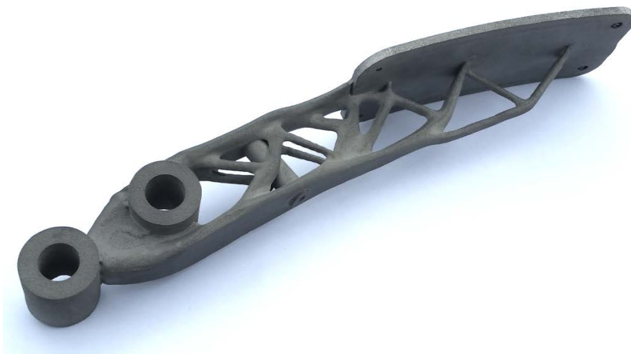
Figure 11: Manufactured topology optimised brake pedal with lattice designed foot pad.
