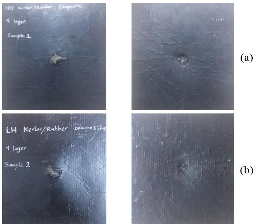
Fig. 14 Front and back face of rubber matrix composite after perforation (a) HH rubber matrix composite (b) LH rubber matrix composite
