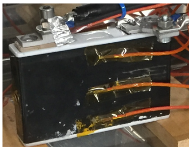
Fig. 7 Cell Thermocouple Test Setup
