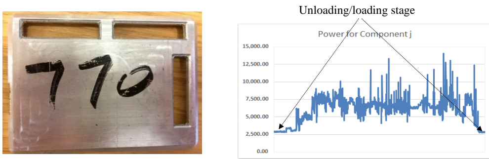
Figure 8: Energy consumption monitored during the unloading/loading stages.
