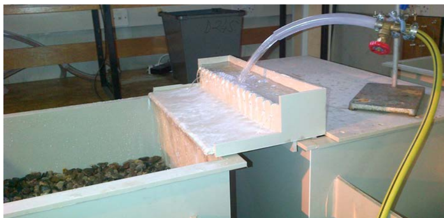
Figure 2 - Spillway in operation
