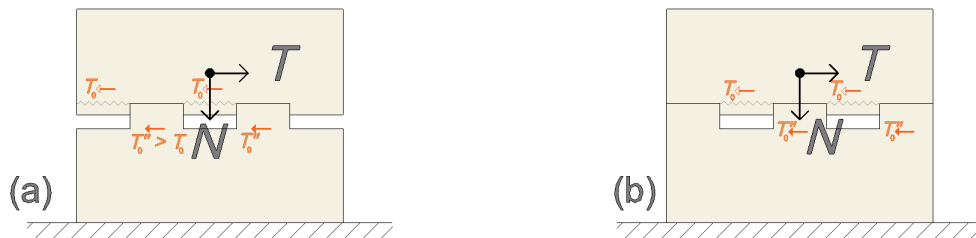
Figure 5. Sliding resistances of interlocking blocks with lower connectors higher than upper ones (Case 3).
