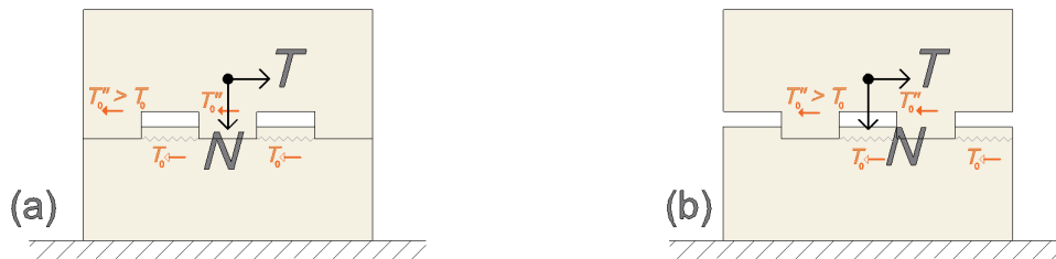
Figure 4. Sliding resistances of interlocking blocks with upper connectors higher than lower ones (Case 2).
