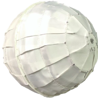
Figure 19. Probe sphere wrapped in sewn Beta cloth.
