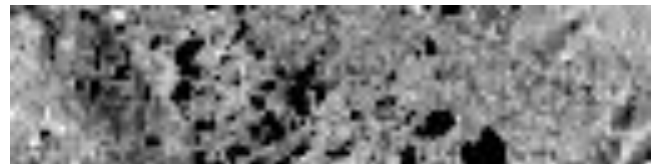
Fig. 4. The simulated VIIRS subset corresponding to the VIIRS subimage displayed in Fig. 1, created by convolving the resampled Landsat OLI image (as in Fig. 3) with the VIIRS PSF (as in Fig. 2).
