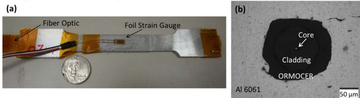
Figure 3. Embedded fiber optic strain sensors: (a) ASTM tensile sample used to evaluate strain sensing performance; (b) micrograph of representative consolidated fiber showing metal completely encapsulating the fiber.
