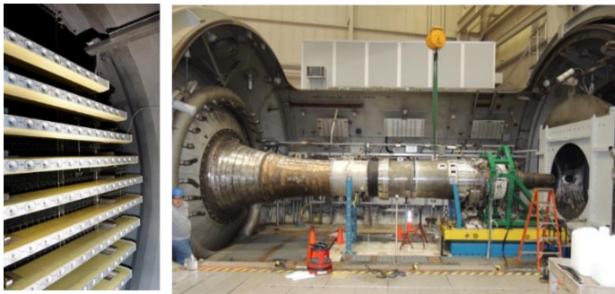
Figure 1. Engine Testing in PSL at Simulated Altitude and ice crystals. Direct connect duct (right), spray bars (left).
