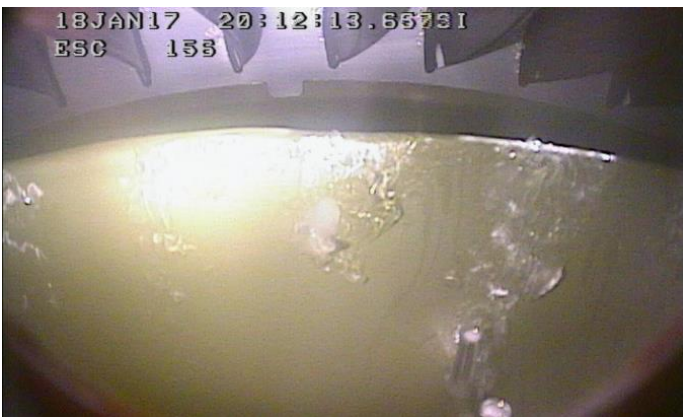
Figure 13. For Escort 156, there was ice accretion on the shroud, without horns on the splitter-lip.
