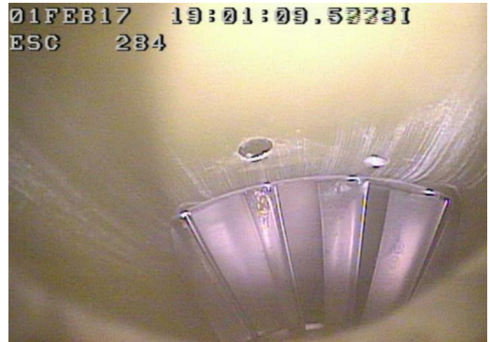
Figure 17. Ice accretion on the IGV surface near the tip (Escort 284 at 36K ft altitude).
