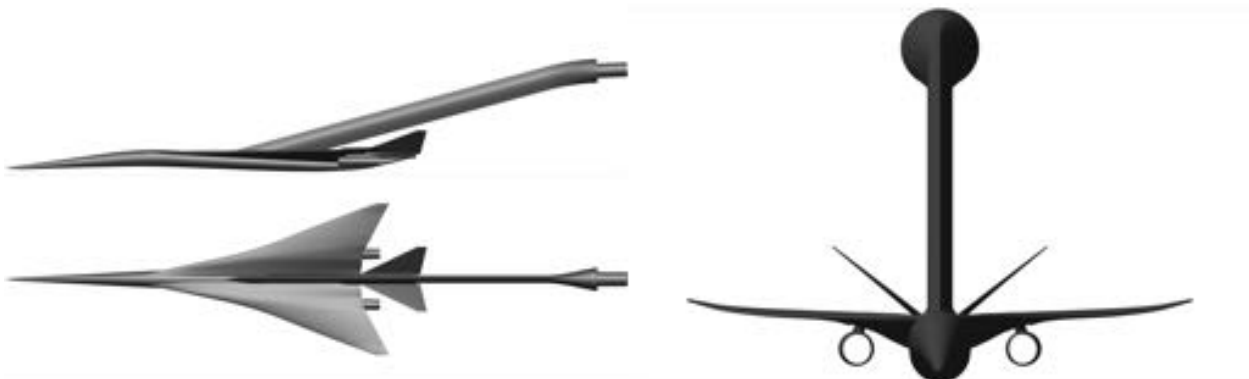
Figure 28. Three-view of the Lockheed Martin 1021 wind tunnel test article.
