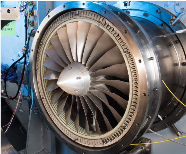
FIGURE 2: R4 TURBOFAN ROTOR INSTALLED IN W-8 WITH TREATMENTS INSTALLED OVER-THE-ROTOR.
