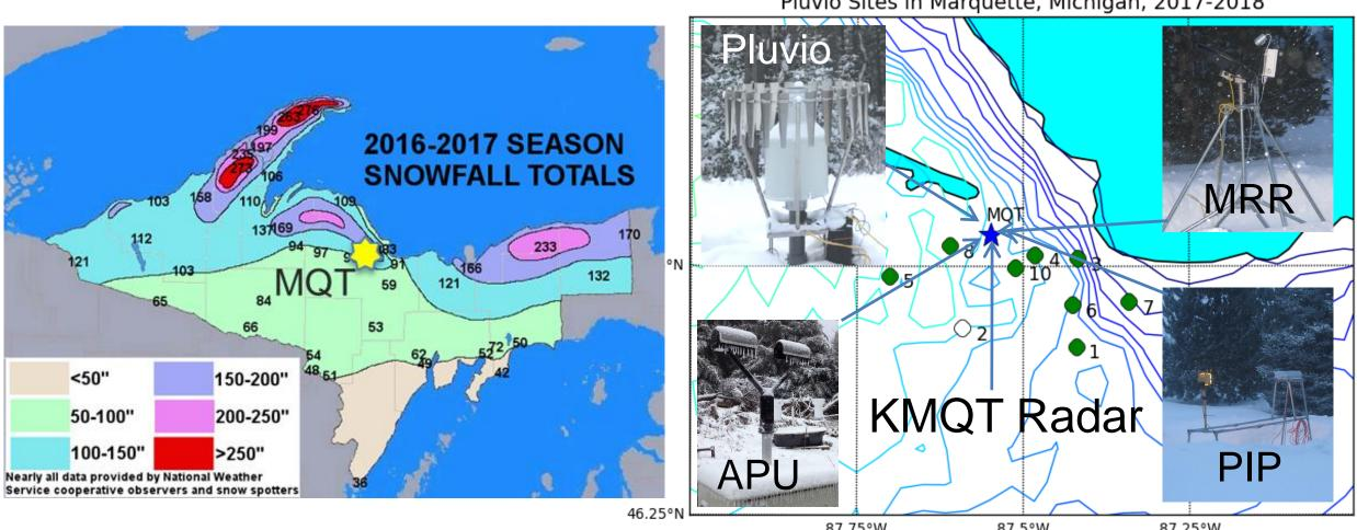
MQT RPN: Pluvio gauges (green dots) SWER "reference" sampling of KMQT estimators; Physics instruments located at MQT,
