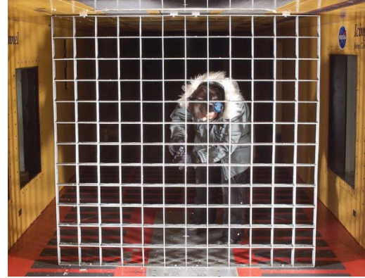
Figure 2.—Technician measuring the thickness of ice accreted on the Grid.
