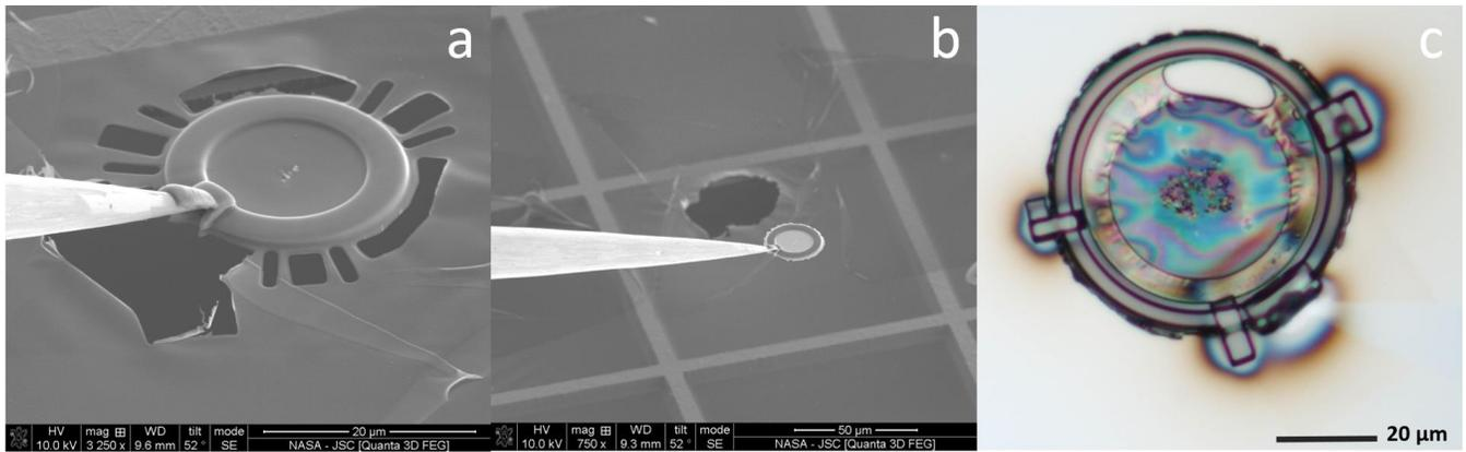
**Figure 1.** a) thin section with deposited C-ring attached to the needle. b) assembly lifted from the C film TEM grid. c) reflected light image of the extracted section attached to a Si substrate for analysis.
