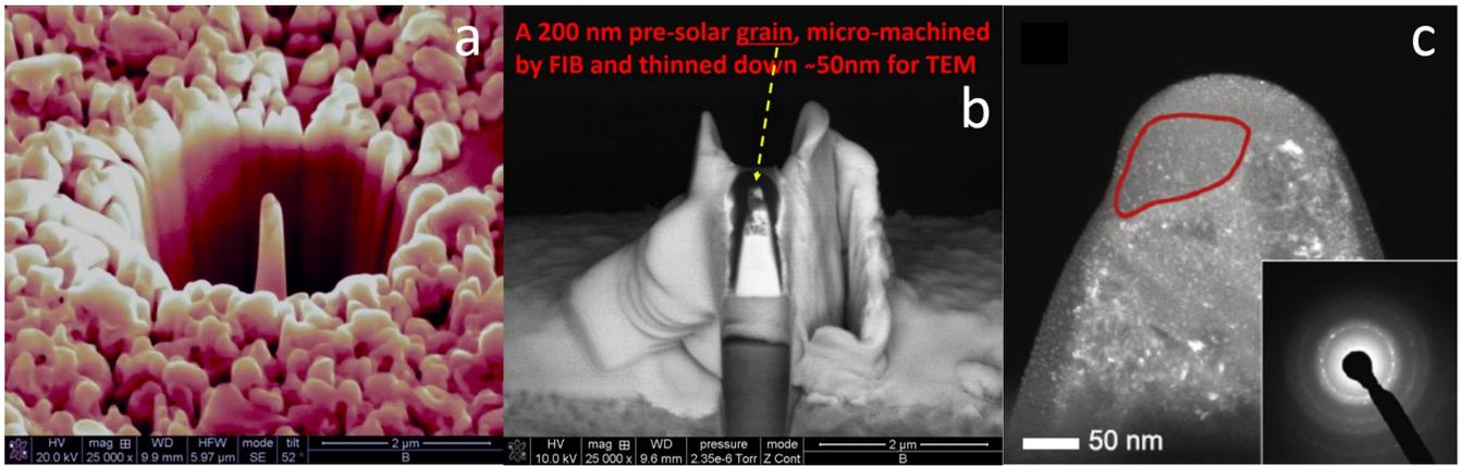
**Figure 2.** a) a sub- $\mu\text{m}$  presolar grain is isolated from neighboring meteorite matrix grains by FIB milling for subsequent NanoSIMS isotopic analysis. b) an electron transparent section of the grain was then produced by FIB for mineralogical analysis by TEM. c) darkfield TEM image and diffraction pattern from the presolar grain [3].
