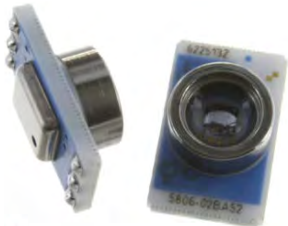
Fig. 31. The MS5806-02BA miniature altimeter from Measurement Specialties (Fremont, California) is a very small ( 6.4 \times 4 \times 2.8 \text{ mm}^3 ) lightweight (0.14 g) device with very low power consumption (1.4 mA at 3 VDC, peak) spanning a wide operating temperature ( -40 to 85^\circ\text{C} ).
