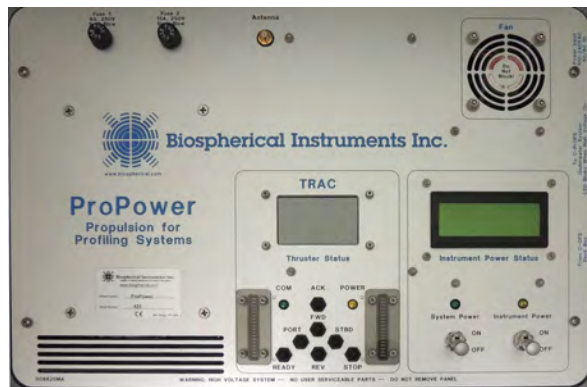
Fig. 37. The ProPower box panel showing the TRAC components (lower middle), and the LCD display for instrument power status (lower right) above the system and instrument power switches.
