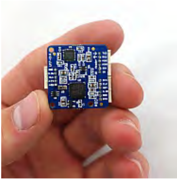
Fig. 32. The UM7 orientation sensor from CH Robotics (Payson, Utah) is a comparatively very small ( 27 \times 26 \times 6.5 \text{ mm}^3 ) lightweight (11 g) device with low power consumption (50 mA at 5 VDC) and a wide operating temperature ( -40 to 85^\circ\text{C} ).
