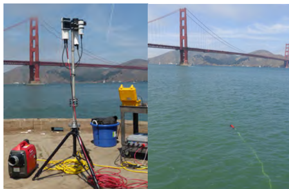
Fig. 24. The deployment of a C-OPS using the C-PrOPS and C-CAPS accessories from Torpedo Wharf near the Golden Gate Bridge in San Francisco Bay, wherein the reference and support equipment (left) are shown with the profiler (right).
