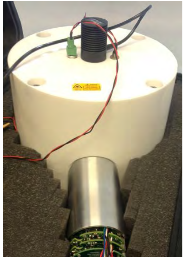
Fig. 45. An early version of the OCULLAR prototype radiometer (contained principally within the silver cylinder) with exposed support electronics boards (green) and mounted in the lineator (white). The foam (gray) provides insulation for temperature stability and support for the prototype.
