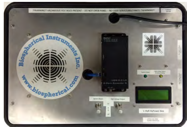
Fig. 30. The prototype HyPower box developed for the C-HyR profiling accessory, wherein the USB extender is the black rectangular box in the middle is the USB-to-Ethernet extender and the cable exiting above is the 120 VAC power cable used to supply power to the box.
