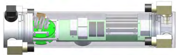
Fig. 14. A transparent drawing of the C-PrOPS electronics module that also contains the PCA for the CT sensor.
