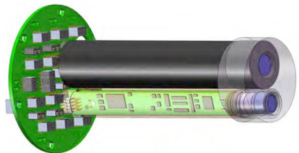
Fig. 50. A drawing of the new PMT microradiometer (dark gray) paired to a standard SiP microradiometer (light green). The PCA with integral HV control and digitization (dark green) for mounting the PMT-SiP microradiometers is redesigned both for added functionality and packing efficiency.
