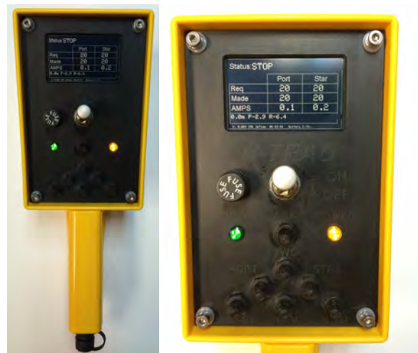
Fig. 36. The handheld C-TRAC developed for the C-HyR profiler (left) and a close up of the display and controls (right).
