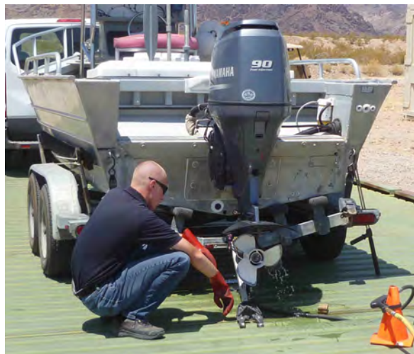
Fig. 65. Decontamination of the outboard motor cooling system after recovery of the R/V Hobson’s Choice at Lake Mead (Nevada).
