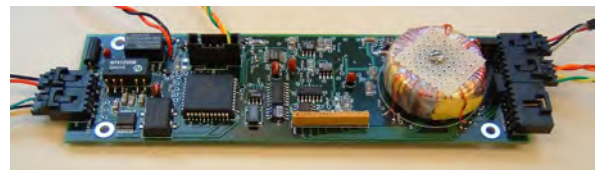
Fig. 15. The PCA for the CT sensor, which is mounted inside the electronics module.
