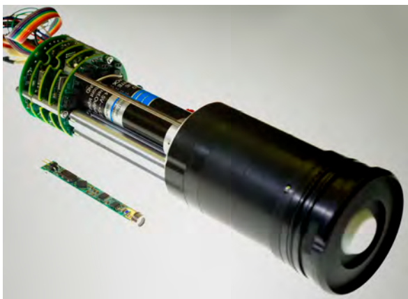
Fig. 44. The OCULLAR prototype irradiance instrument without the external housing (right) next to a SiP microradiometer (left). The two PMTs (black with silver and blue labels) are above the microradiometers, which are in aluminum (silver) sleeves.
