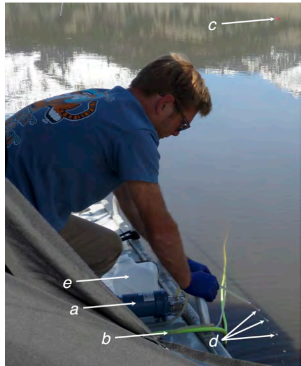
Fig. 63. The C-PUMPS accessory in use as part of small-boat operations on the shore of Little Lake Washoe showing the following: a) the peristaltic pump; b) the tubing attached to a C-OPS with C-PrOPS sea cable; c) the profiler at the surface far from shore; d) the discharge from the pump; and e) the collapsible sample container.
