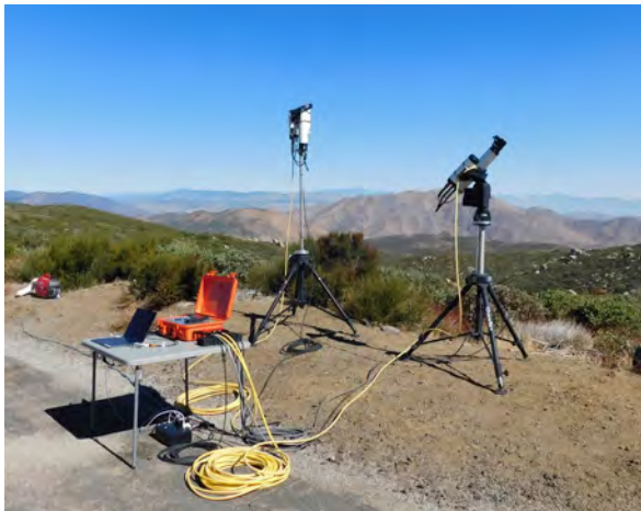
Fig. 104. The C-OSPRey instrument suite mobilized on Mount Laguna for a Langley calibration. Power is supplied by a generator (red) connected to a small UPS below the table supporting the acquisition computer and a HyPower box with two cable ports (HyPower2) and advanced capabilities denoted the HyPower2+ (orange).
