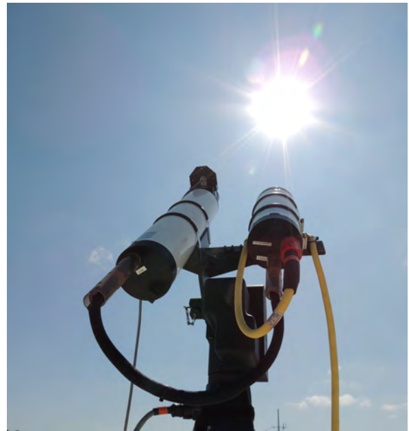
Fig. 103. The C-OSPRey radiance instrument (right) mounted on the PTU-D300 with the ERA and quad detector (left) tracking the Sun as part of observing the August 2017 solar eclipse.
