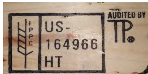
Fig. 106. The IPPC mark on one of the SV3 shipping crates; all marks are preserved with two-part clear marine epoxy.
