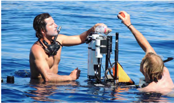
Fig. 101. The at-sea cleaning of the C-PHIRE solar reference on the SV3, which is recorded for detailed observations.
