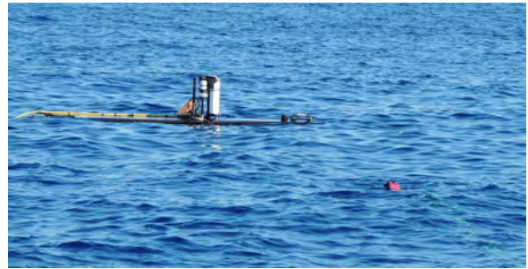
Fig. 102. The system 21 C-OPS with C-PrOPS accessory (foreground) being steered with digital thrusters towards the SV3 (background).
