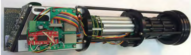
Fig. 119. The internal assembly of the C-OSPREy radiance radiometer from right to left, as follows: (black) gershun tubes, (silver) microradiometer array and filter wheel (colored wires visible), and (green) support electronics with CGS behind (partially visible).
