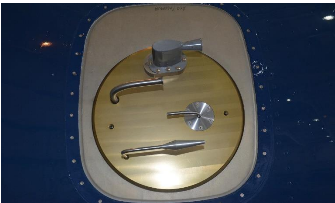
Figure 21. BHS Inlets and solid wire TAT on window blank (station 530)
