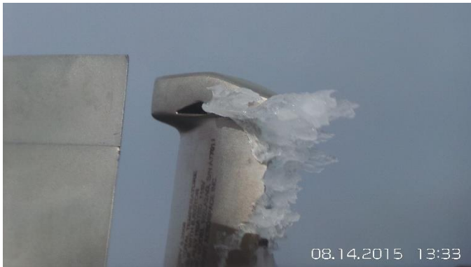
Figure 17. Ice on backside of TAT probe after flight in HIWC
