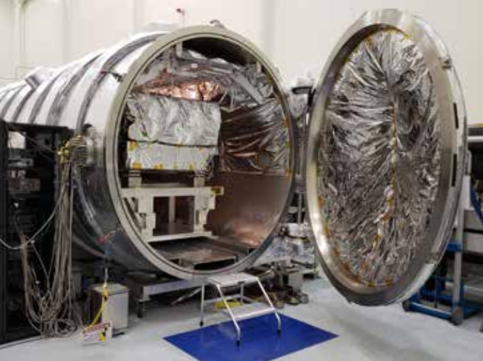
▶ Left: The Decadal Survey Testbed inside the vacuum chamber at the High Contrast Testbed Facility at the NASA Jet Propulsion Laboratory (JPL). Right: Manager of the testbed facility, Dr. Camilo Mejia Prada, looks into the vacuum chamber to view an ongoing coronagraph experiment.
