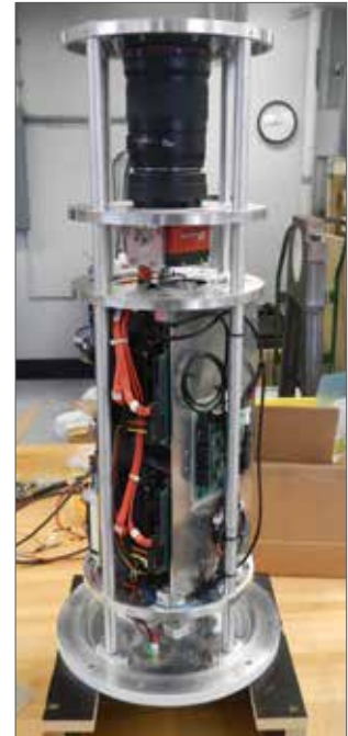
▶ PMC turbo pressure vessel imaging system components: lens, camera, computer and data storage.
