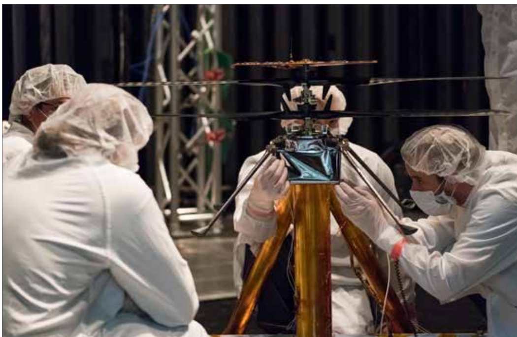
► Members of the Mars Helicopter team preparing the helicopter for a test in the Twenty-Five-Foot Space Simulator.
