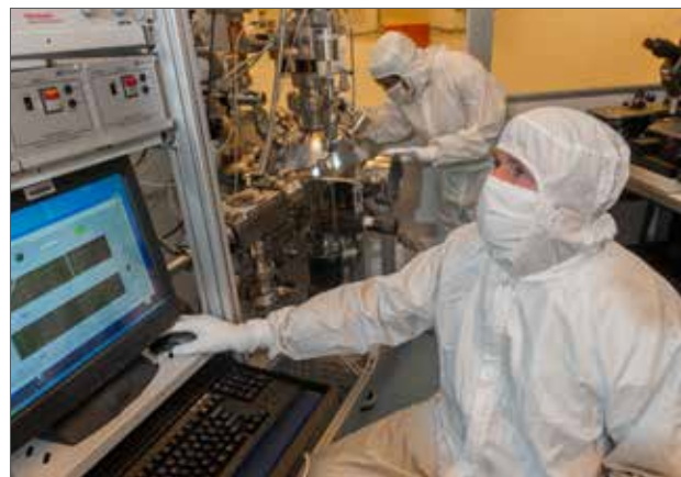
▶ SiC IC Memory Team members depositing chip interconnect metal in the NASA GRC Microsystems Fabrication Laboratory.
