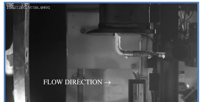
Figure 6. Picture of ice accreted on the RFP body positioned just downstream of the PSL exit duct.
