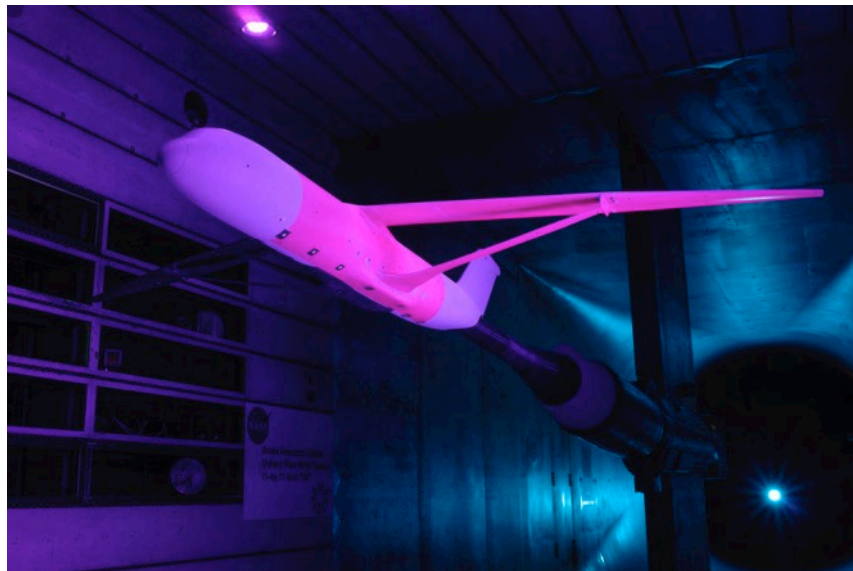
Figure 7. TBW Model with PSP Installed at 11-by 11-foot Transonic Test Section
