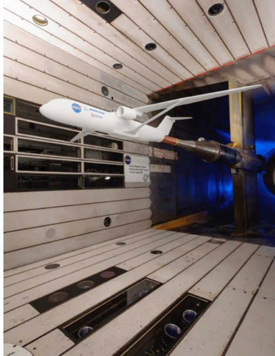
Figure 4. NASA / Boeing Truss Braced Wing Model Installed in the 11-by 11-foot Test Section
