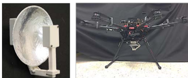
Figure 3. Sensor-mirror UV detector and vehicle mounting. A dish with 12.7 cm (5 inch) diameter and 0.35 focal ratio (left) provided the desired 6.1m (20 ft) range over a 16° half-power beamwidth. For mechanical stability, additional support struts and an angled sensor arm were used in the detector mounted on the UAV (right).
