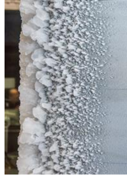
Figure 7. Photograph of leading edge ice accretion on a 72-inch chord NACA23012 airfoil. Suction Surface. Test number EG2819.
