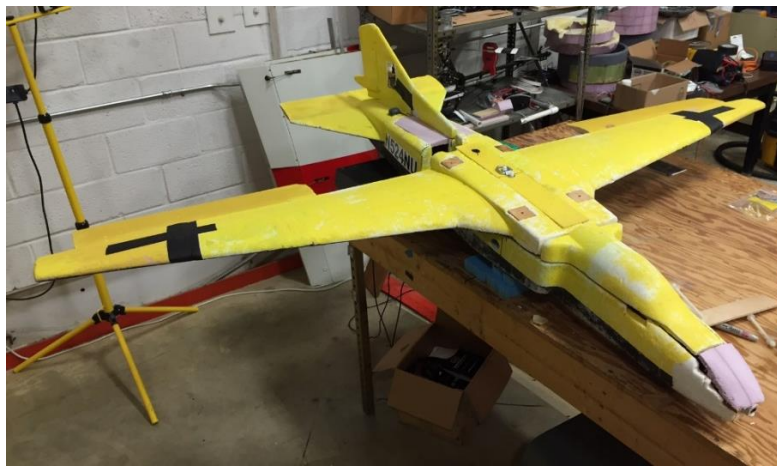
Fig. 5 “Foamy” airframe during a control surface test.
