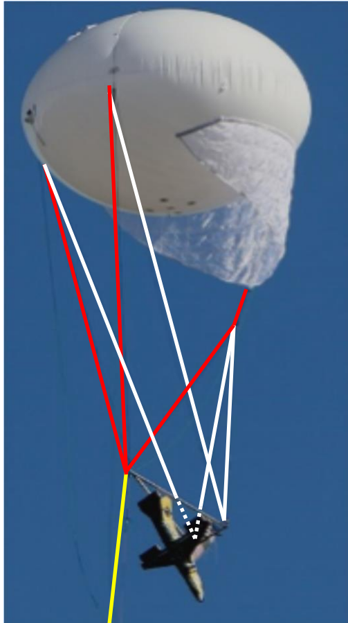
Fig. 1 Line configuration. Tether (yellow), load-bearing suspension lines (red), supporting suspension lines (white).
