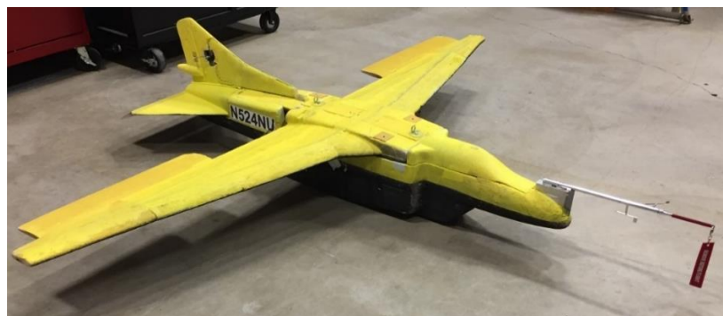
Fig. 6 “Super Guppy Foamy” airframe incorporates a belly extension to house the production Learn-to-Fly avionics.
