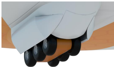
Fig. 12 Illustration of pod gear concept with toboggan.
