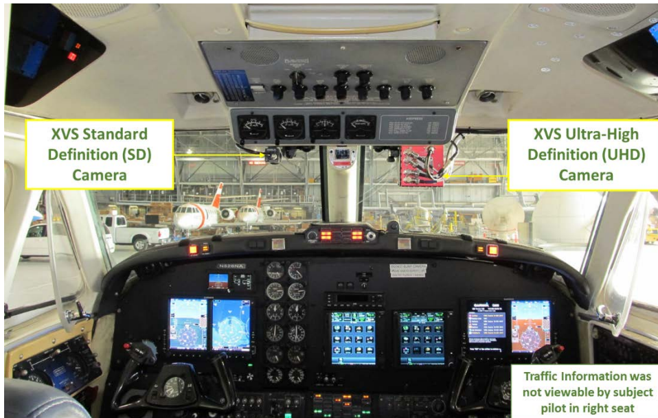
Fig. 2 XVS Cameras mounted in Forward Window
