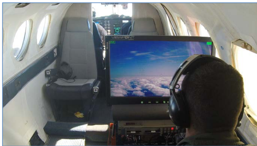
Fig. 3 Over-the-shoulder view of XVS Monitor installation in Cabin
