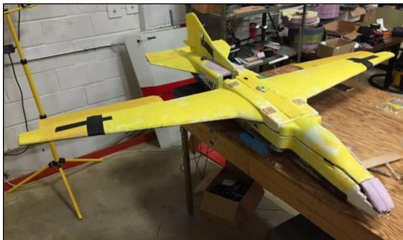
Fig. 3 Foamie glider aircraft used for early L2F concept development.
