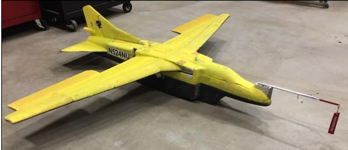
Fig. 4 Super Guppy Foamie glider used for avionics testing.
