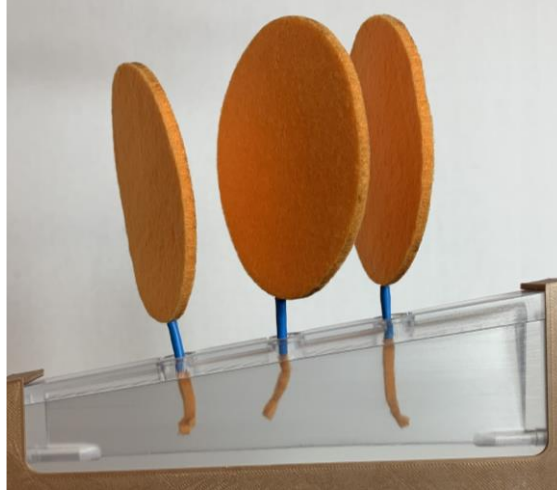
Figure 2. Low-g representation of 3D printed Acura 60 test cell and three rayon felt tap root plant models.
