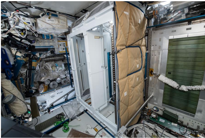
Figure 10. Toilet Stall deployed in ISS Node 3.
