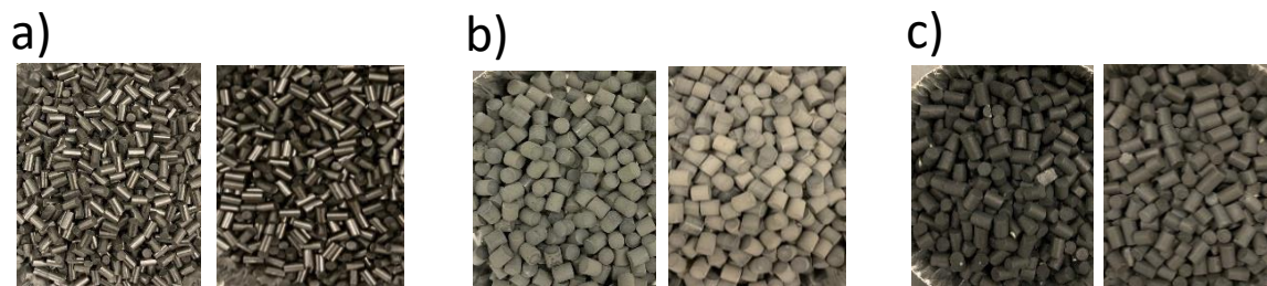
Figure 10: Catalyst pellets before (left) and after (right) chemical contamination test for a) SNG 8000 catalyst, b) 0.5% Ru catalyst, and c) 2.0% Ru catalyst
