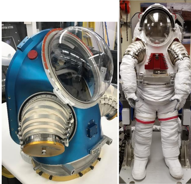
Figure 7: Z-2.5 xEMU Demo configuration
