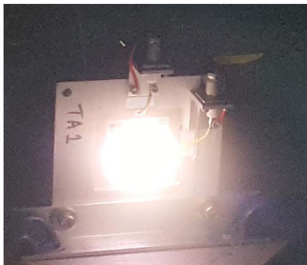
Figure 7. Test article 1 of the LTCC-ET prototype with an RF-driven argon plasma.
