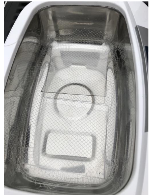
Fig. 7. Two Glass Superstrate Lenses in Ultrasonic Solvent Bath. basket provides easy handling of the thin lenses to avoid cracking the thin glass superstrates.
