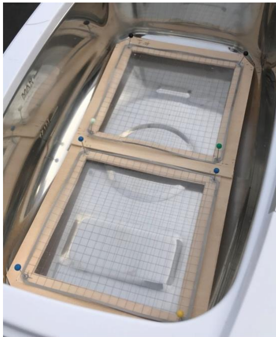
Fig. 9. Two Silicone Lenses with Embedded Titanium Mesh in Ultrasonic Solvent Bath.
