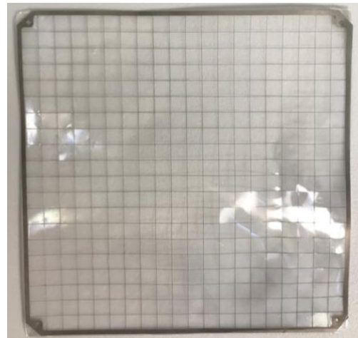
Fig. 10. Embedded Mesh Lens After Dissolving Tool.
