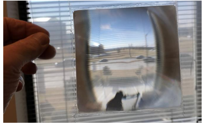
Fig. 6. Polymer Molding Tool Made from Electroform.
